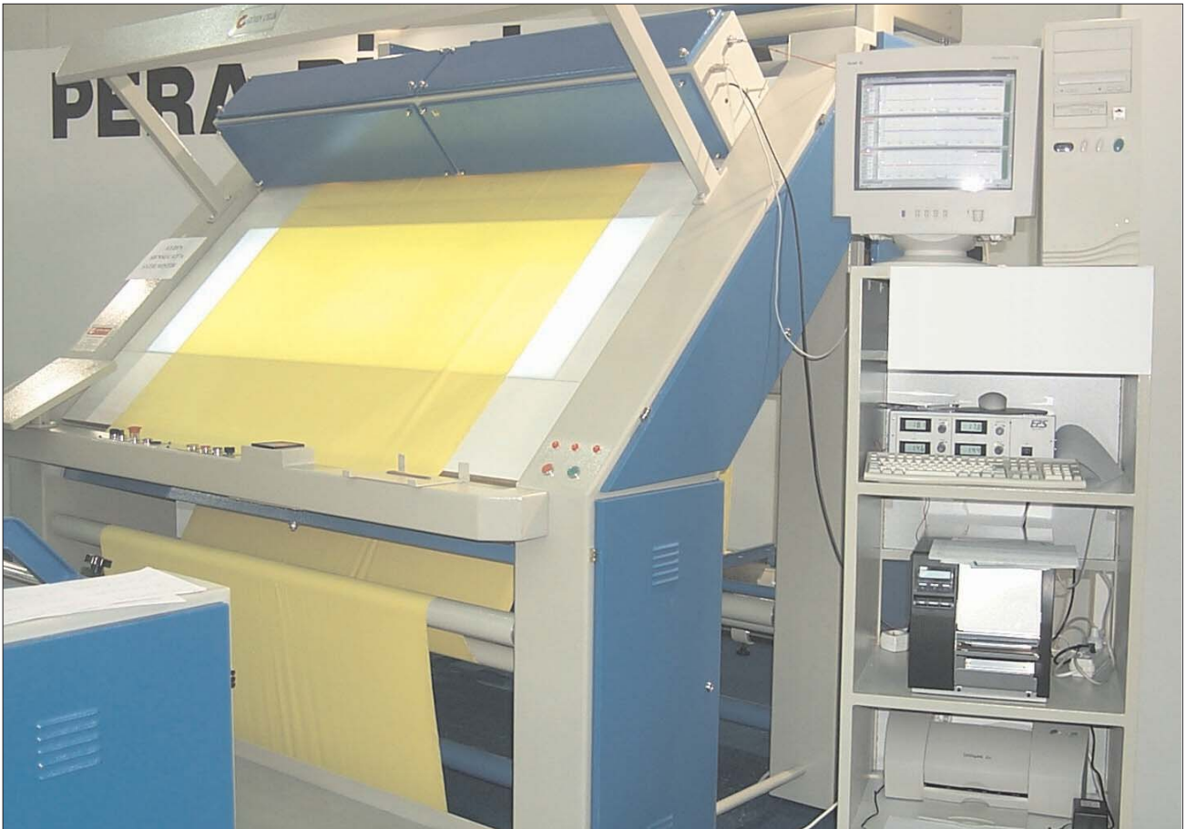
Figure 1. Online spectral / color control in textile dyeing.
