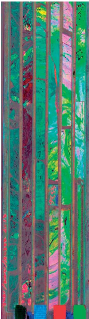
Geologically classified SWIR image of a drill core tray. Image collected in a high speed mode with 2 mm resolution. Tray size 132 x 40 cm, image size 1 050 x 320 pixels.
