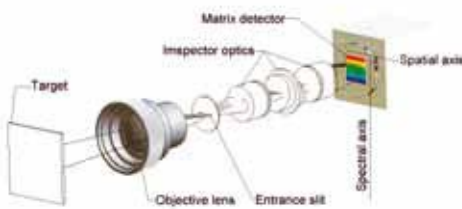
Principle of Spectral Camera
