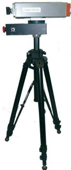
Spectral Camera PS mounted on a rotary stage on top of a tripod
